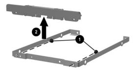
Removing the Hard Drive Upper Bezel
